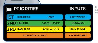
We understand heating systems. We've been leading the industry for close to 150 years. Different types of systems operate at different temperatures, and a home may have a combination of systems in it. We've simplified that too. Our boiler control can send out different temperatures to match the home's systems, assign a priority of what need is met first, and identify what part of the home is set up on
